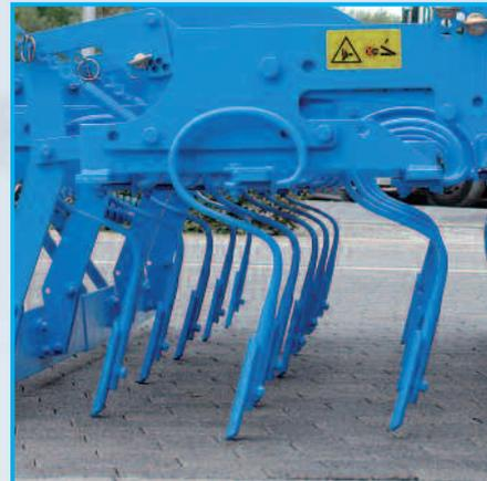
The large number of tine frames available offers the right tools to tackle differing soil and operational conditions. All the tine frames can be rapidly adjusted for depth in fine graduations and without tools. The choice includes harrow frames with marathon tines in two rows or a three-row pattern of gamma spring tines with shares. Frames with duck-foot shares can be ordered in two-row frames.
