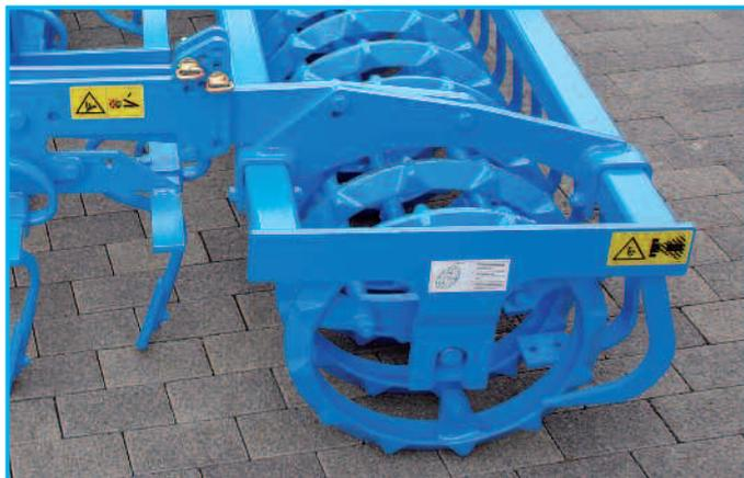
Tine penetration to working depth is controlled by the following rollers. Adjustment of working depth is carried out in fine graduations via hole bar and pin. And always available is the correct type of following implement according to soil type and working conditions. As well as the standard 540 mm diameter tube bar rollers, toothed packer rollers and a range of trapeze rollers are also available.
