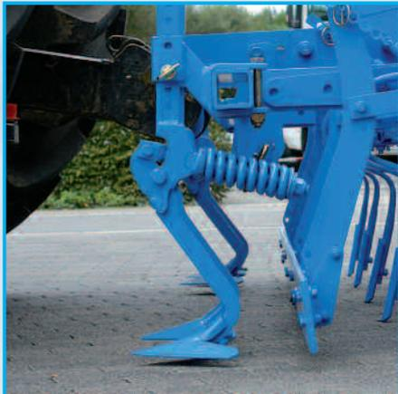
The track looseners can be fitted with either wing or narrow shares and can be easily adjusted in fine graduations to desired working depth. The standard-equipment automatic overload protection is an effective way of avoiding damage. Simply moving them along the square profile frame slides the track looseners into the right positions for any track or tyre width.
