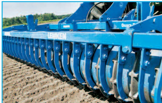
The optimum preparation for sowing is offered by trapeze rollers when used in combination with the drill. These rollers are on offer as various versions and they all help create the very best conditions for good emergence. For intensive crumbling effect and precise strips of reconsolidation before the drill coulters, a choice of 500 mm diameter trapeze ring, packer or disc rollers is available.
